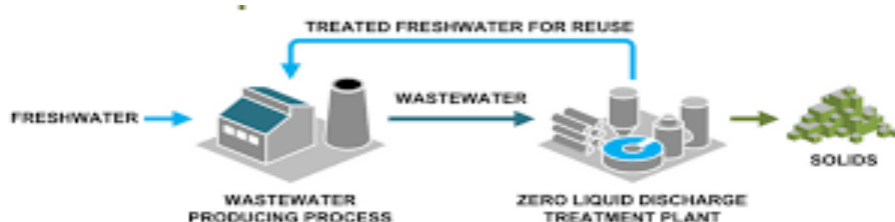
Fig 1.1 Zero Liquid Discharge Process Flow Ref: austrowatertech.com
