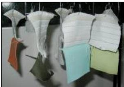
Fig 1.1 Testing specimen for washing fastness test
