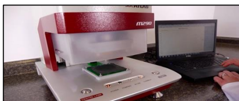
Fig 1.2 Moisture Management Tester
