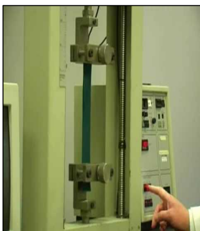
Fig 1.1 – Fabric Tensile strength Test machine
